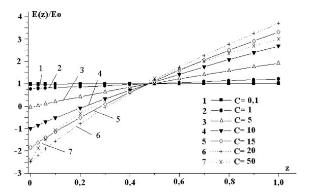
*Puc. 3. Зависимость*  $E(z)/E_0$  *om* z = x/l *npu*  $\gamma = 1$   $(E_0 = 5.8 \cdot 10^7 \text{ B/m}).$
