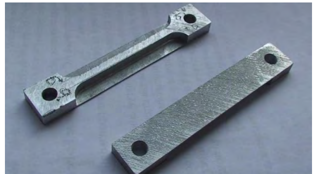
Fig. 2. Specimens for the coating. On the right - metal block blank for specimen, on the left - specimen ready for ESA.
