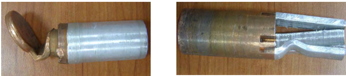
Fig. 6. Macroscopic images of the Al alloy/ Cu friction welded samples.
