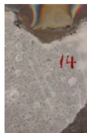
Fig. 10b. The surface morphology of MAO coating after treatment 14 s (NaOH: 0.02 mol/L).
