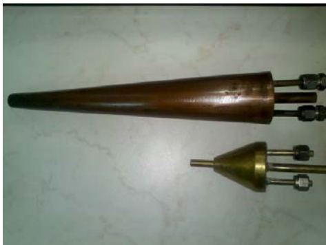
Fig. 2. Photographs of new and previous designed cold fingers. The length ratio of the new cold finger vs. an older design is over 4.5:1.
